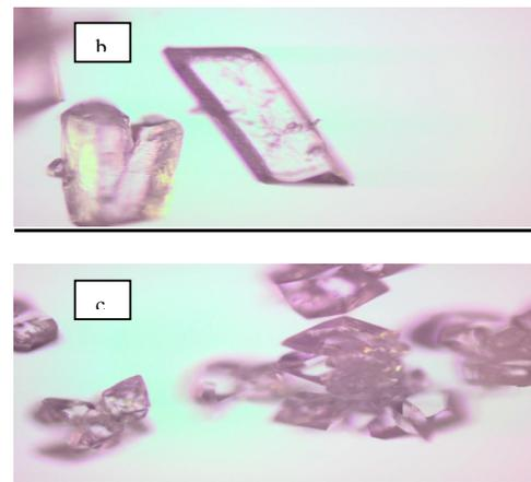
**Figure 2:** (a) Plot of FBRM fine counts against the constant relative supersaturation used for each control experiment, also included in this figure is the median ( $\mu\text{m}$ ) plotted against the constant relative supersaturation. Shown on the right hand side (b and c) are two microscopic pictures of paracetamol crystals obtained from two control experiments, 0.003 (Top) and 0.009 (Bottom).
