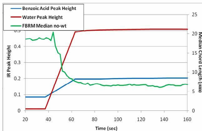
**Figure 3:** Tracking attainment of steady state using IR supersaturation peak heights<sup>1</sup> and FBRM no-wt mean
