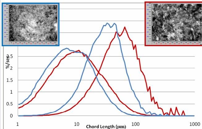
**Figure 2:** FBRM CLDs and PVM images for high (1:2) and low (9:5) feed : anti-solvent flow rate ratios
