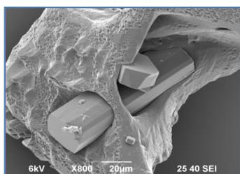
Figure 1 SEM image of FV crystal undergoing a solution mediated polymorphic transformation to FII and FIV. Mother crystal FV is observed to be dissolving (pitted surface) as the new polymorphs FII and FIV grow into the mother crystal. Experiment was carried out at 10°C in Ethanol.
