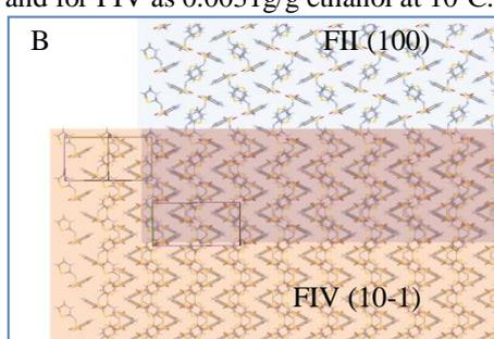
Figure 2 (A) Scanning Electron Micrographs of FII Sulphathiazole crystals exhibiting the characteristic inclusion in the centre of the crystal and (B) Mercury 2.2 representation of the molecular packing in FII and FIV Sulphathiazole viewed from the proposed faces in contact showing how the structures align. The (100) face in FII is highlighted in blue and (10-1) face in FIV is highlighted in red. The overlapping zone is highlighted in purple.
